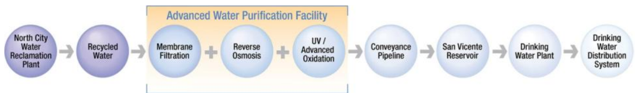
Figure A - 4: Components of a Multiple Barrier Reservoir Augmentation Project at San Vicente Reservoir
